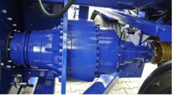
Robust drivetrain with separate gearboxes and replaceable shaft
