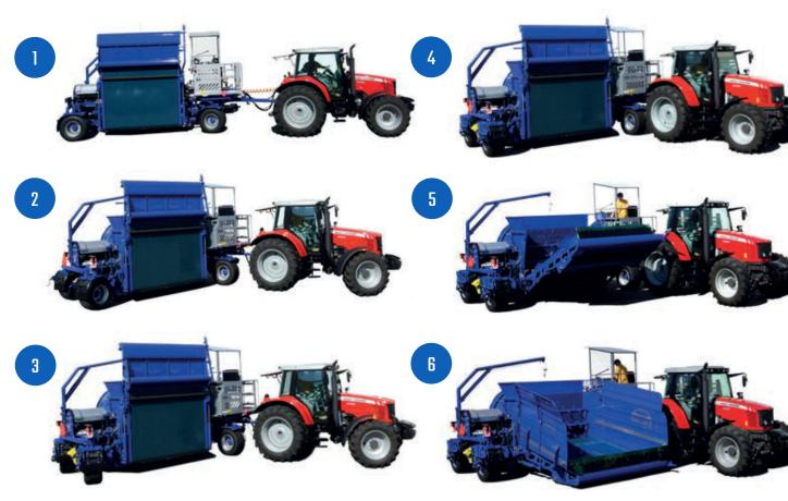
The tractor is attached to the machine at the same point both for both operation and transport. Machine setup after arrival at the work site is much faster and easier compared with other machines.
