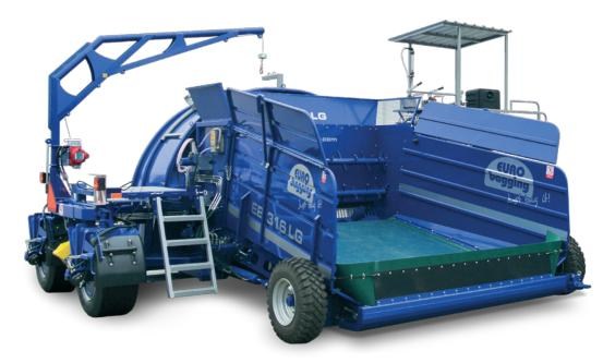
A silage bagger with a large tunnel that makes it capable of storing large amounts of food in bags and is ideal for use in large farms, service businesses, and biogas plants. It is intended for storing grass silage, corn silage, sugarbeet pulp, and CCM. The unique QUICK system allows the machine to be quickly set up into working position. The comfortable hydraulic accessories have proportional main control functions.
